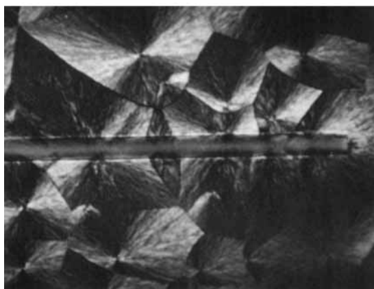
Figure 14 Morphology of model thin PPS film/single glass fiber composites viewed through a polarizing light microscope Magnification: (a) un-sized, 360 \times ; (b) sized, 570 \times .
